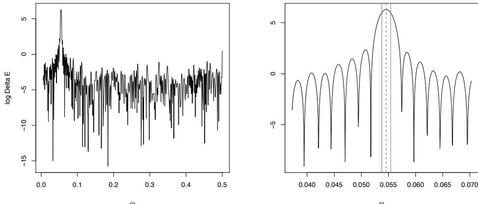
Figure 1: The energy  $\log \Delta E(\omega)$  for a noise level  $\sigma = 0.2$  is shown on the left for a range of frequencies  $\omega$ . A close-up of the region around the peak is shown on the right. The two frequencies  $\omega_1$  and  $\omega_2$  are marked with solid vertical lines, while the *resonance* frequency  $(\omega_1 + \omega_2)/2$  is shown with a broken vertical line.
